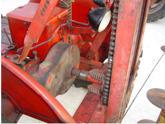
Gear reducer/reverser and chain drive on a Farmall Cub. ©2011, S. Butram, West Lafayette, IN. Used by permission.
