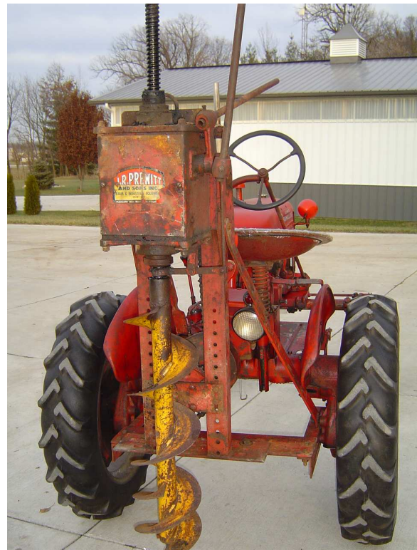
Prewitt Digger mounted via brackets on a Farmall Cub. ©2011, S. Butram, West Lafayette, IN. Used by permission.
