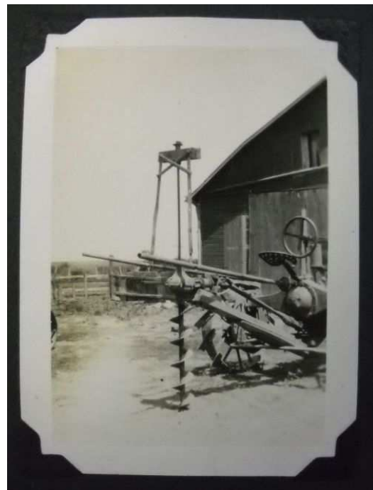
The original 1936 Grosshart Post Hole Digger mounted on a Farmall Regular.
