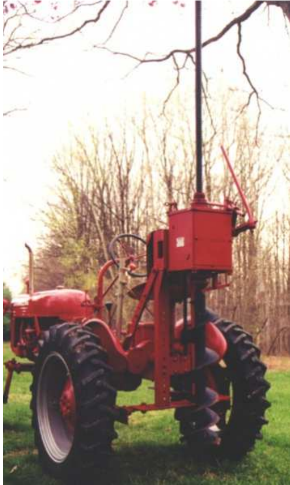
Prewitt Post Hole Digger mounted on an IH Farmall Cub. © 2011, J. Freeland, Parkton, MD, Used by permission.
